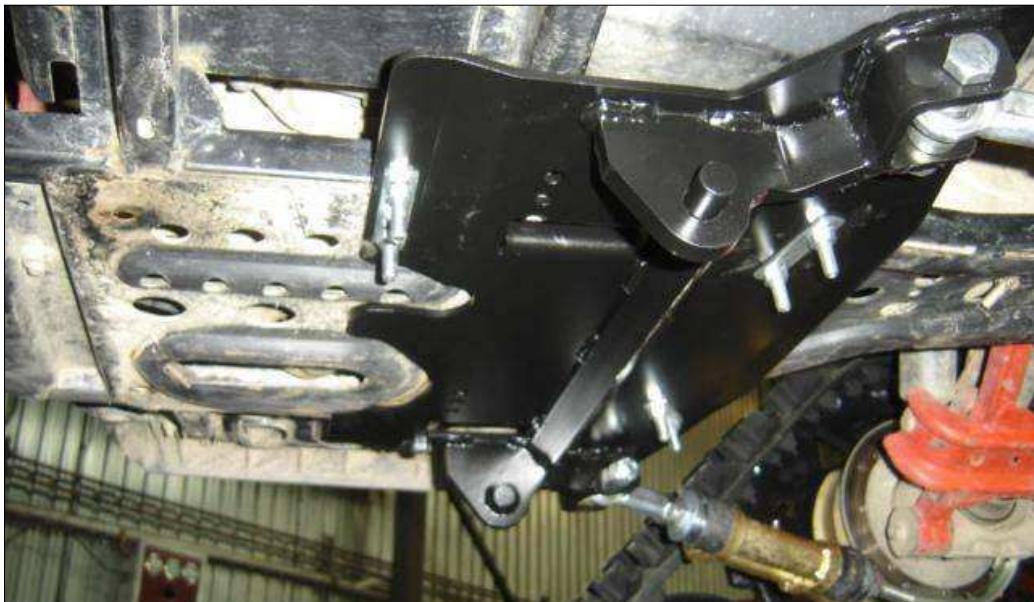
Using the slot as a guide, drill the frame where needed with a 11/32" drill.
