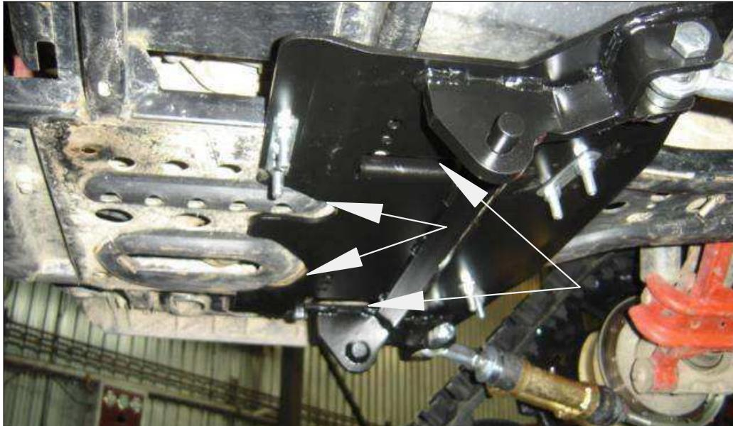
Attach well the plate 03PA-263 to the structure .
