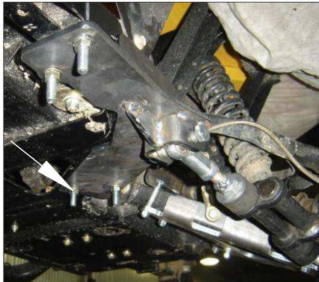
Attach well the plate 03PA-267G to the frame .
