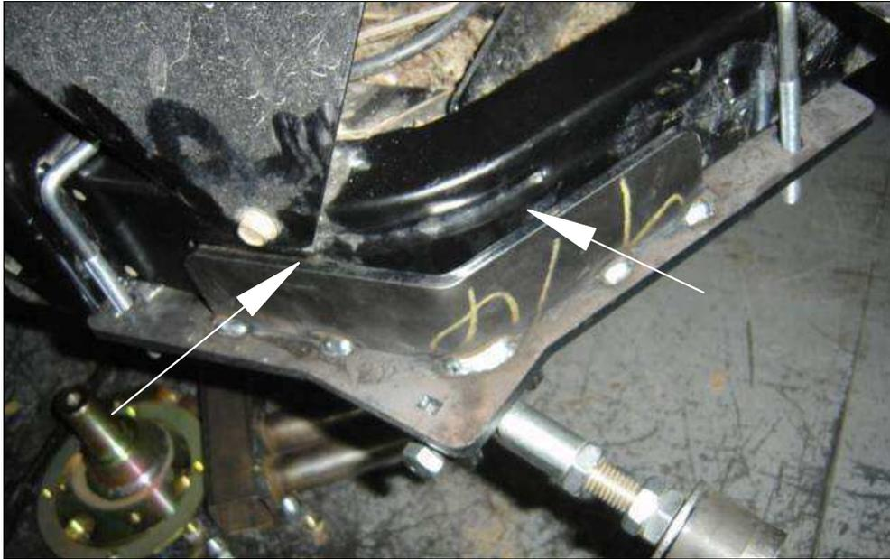
Put the L shaped plate along the frame's corner.
